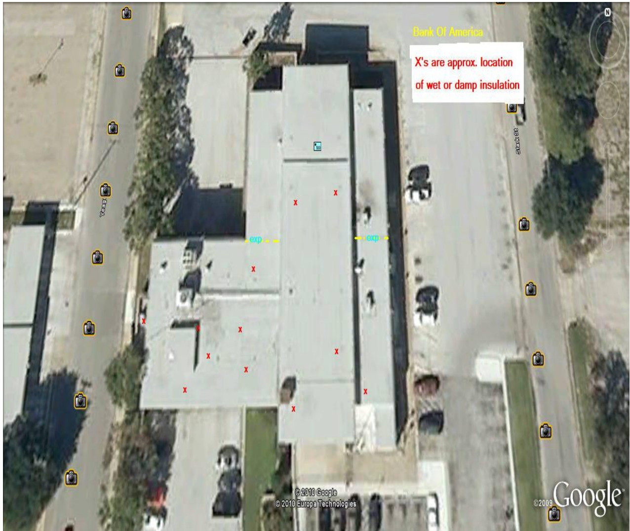
Aerial View Of Roof Marked With X's Indicating Locations Of Wet Insulation
